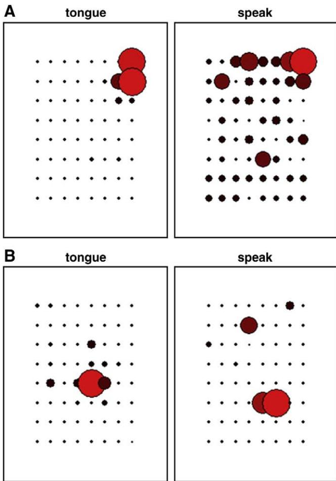
**Fig. 2.** SIGFRIED output. Visual representation of signal correlation with cued tongue motor (left column) and speech (right column) activity for patient A (top) and patient B (bottom). Grid numbering proceeds from left to right and top to bottom such that electrode 1 is at the top left, electrode 8 is at top right, and electrode 48 is at bottom right. Circle size and hue are proportional to the  $r^2$  value for the given task and location.
