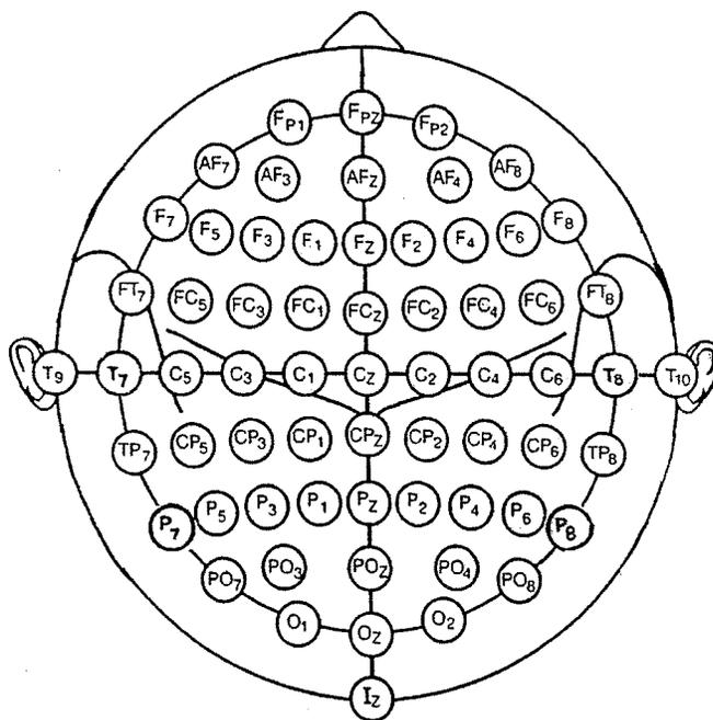
Fig. 3. The standard 64 scalp electrodes (from [15]) used by the laboratory BCI system. The subject's nose is at the top. While only a few electrodes control cursor movement online, activity from all 64 is stored for later analysis. All electrodes are recorded versus an ear reference so that spatial filters can be applied after digitization.
