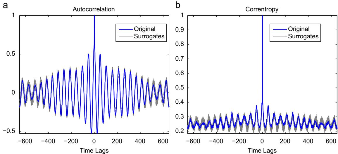
Fig. 9. (a) Autocorrelation and (b) correntropy functions of dataset *E.14* and surrogate series.
