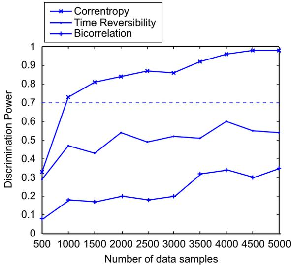
Fig. 4. Discrimination power of the three measures on noisy Lorenz series (SNR = 20 dB) as a function of varying data lengths.
