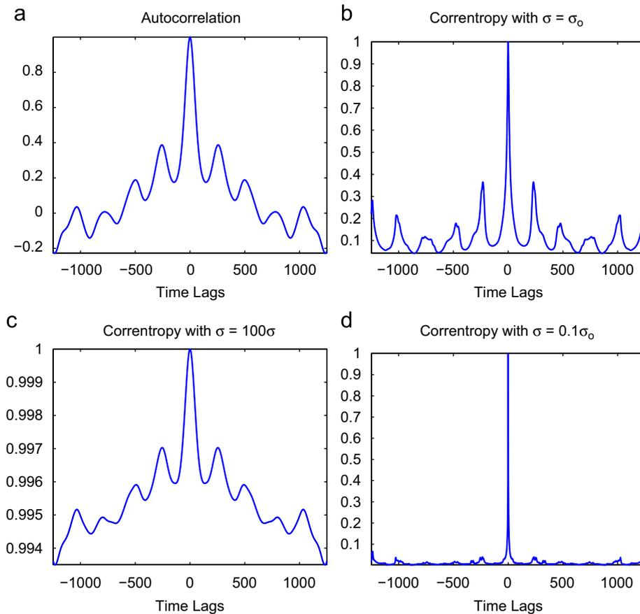
**Fig. 6.** Comparison of autocorrelation and normalized correntropies of Lorenz data with kernel widths  $\sigma_0$  (based on Silverman's rule),  $100\sigma_0$ ,  $0.1\sigma_0$ .
