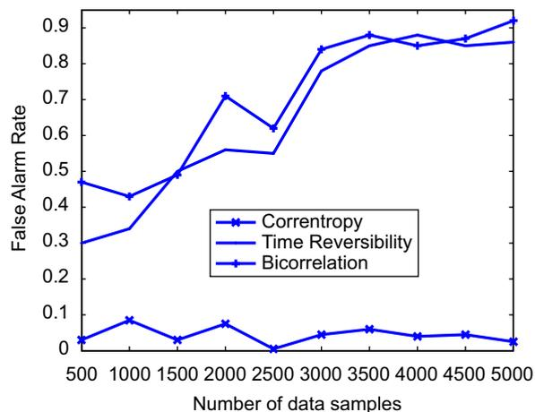
Fig. 2. False alarm rates of the three measures on noisy synthetic linear non-Gaussian data (SNR = 20 dB).
