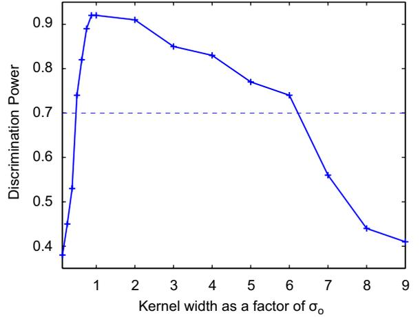
Fig. 5. Discrimination power as function of kernel sizes for the Lorenz series with  $N = 2500$  and (SNR = 20 dB).
