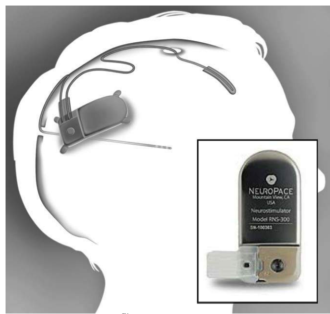
Fig. 22. Photograph of the RNS System neurostimulator and schematic of the neurostimulator sited in the cranium and connected to one depth lead and one subdural strip lead.
